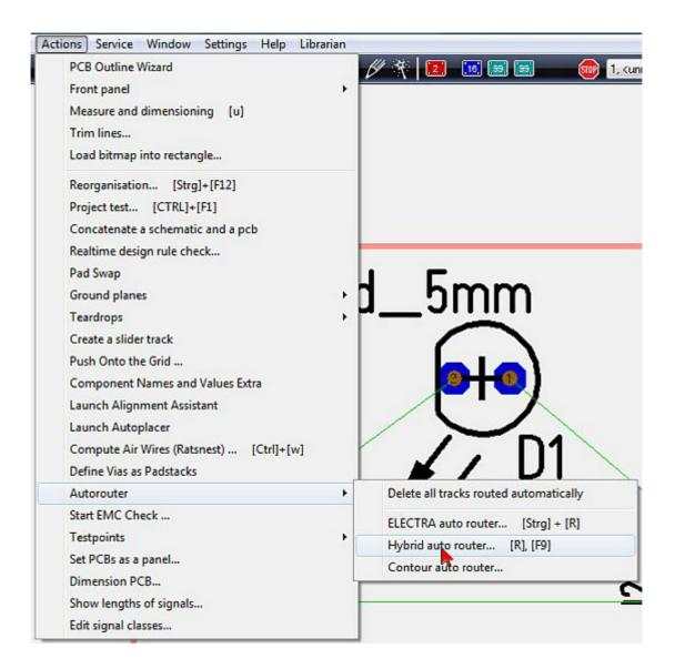
The opening dialog of the hybrid router has three sections divided by tabs. First the section "Signals".
