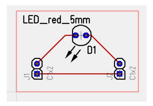
Deletion of the routing result: Drag a highlighting square over all and press the **[Del]** key. Only the autorouted <u>tracks</u> will be deleted.
