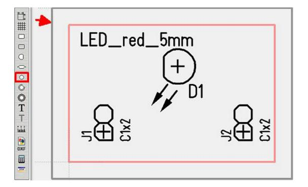
The grey frame is the outline of your front panel. Now tick the icon in order to place a drilling. Alternatively use the Front panel menu option "Place drilling".
