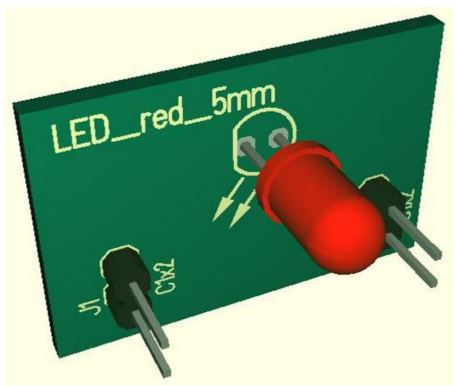
For reasons of computing time the ground plane with it's grid structure on the bottom side is omitted.
