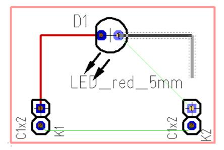
The dashed line which goes along beside the signal line represents a spacing having the the bigger value of both
