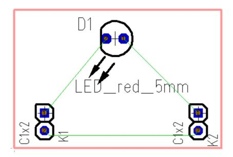
Clicking this icon will let you start Drawing the <u>tracks</u>. Click on a pad and drag the mouse to another pad for creating the connection. Toggle the bending mode by the use of the space bar or use the buttons in the sidebar in section "Settings":
