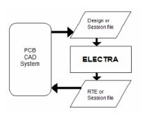
today's complex PCBs. ELECTRA provides immediate feedback on the routing progress and conflict reduction rate.
